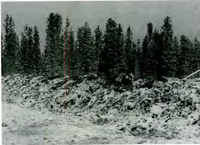
Figure 6-5: Windrow Composting in the Sub-Arctic (note steam coming from top of pile)
